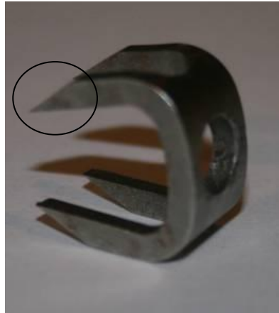
Figure 34. Photograph of an SMA staple. The circle indicates the bevelled staple tip which would facilitate downwards cutting and the staple blade advances forward.
