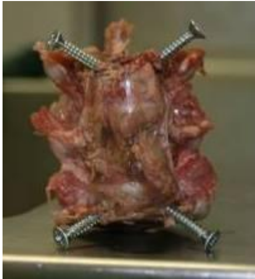
Figure 17. A functional spinal unit following preparation for testing
